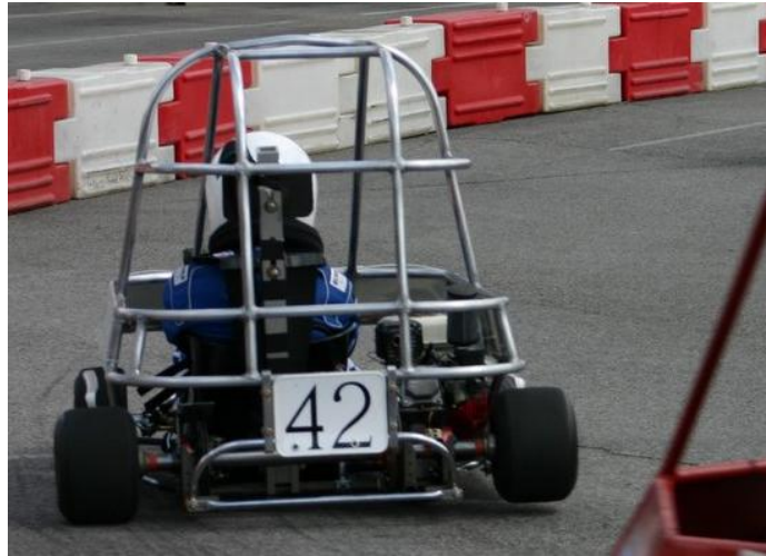
Figure 5: The inside rear wheel is lifted to compensate for the lack of a differential.
