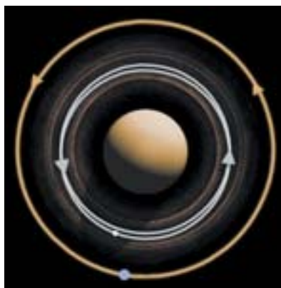
RESONANCE between a satellite and a ring particle means that their two orbits are choreographed: in this case, the particle goes around exactly twice in the time it takes the satellite to trundle around once. Because the bodies always encounter each other at the same position, gravitational tugs can add up.
