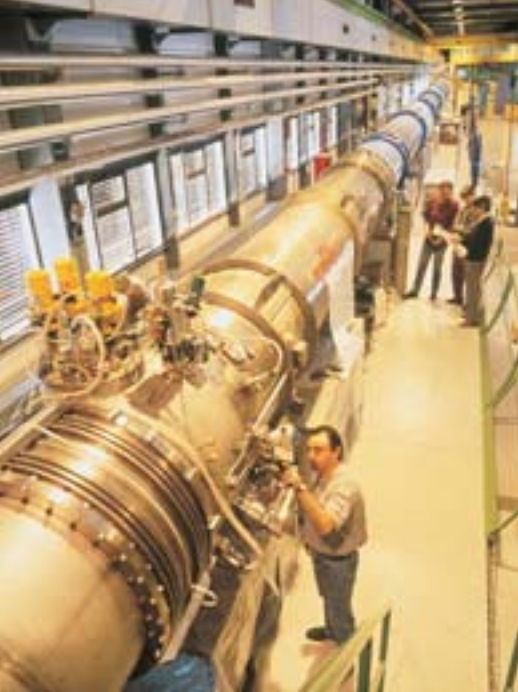
SUPERCONDUCTING MAGNET test string is laid out in the assembly hall; 1,232 large magnets will bend the trajectory of the two proton beams to follow the curve of the accelerator's tunnel.
