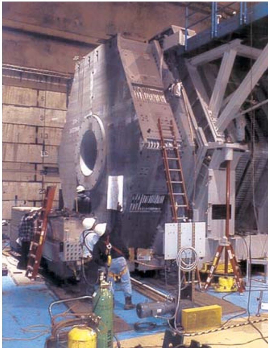
BABAR DETECTOR at Stanford University, built by a collaboration from nine nations, is designed to capture the decays of B mesons in charge-parity studies.
